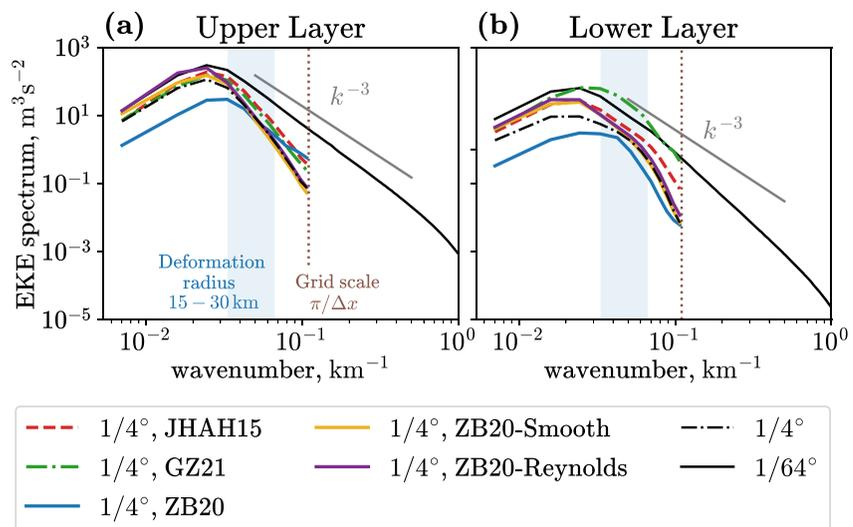
**Figure 2.** The eddy kinetic energy spatial spectrum as a function of wavenumbers for the last 10 years of the simulation: (a) upper layer, (b) lower layer. The unparameterized model (1/4°, dotted dashed line) is compared to parameterized models (JHAH15 in red, GZ21 in green, ZB20 in blue, ZB20-Smooth in yellow, ZB20-Reynolds in violet) and high-resolution simulation (1/64°, black line). The spectrum is computed in the region indicated by the white rectangle in Figure 1.
