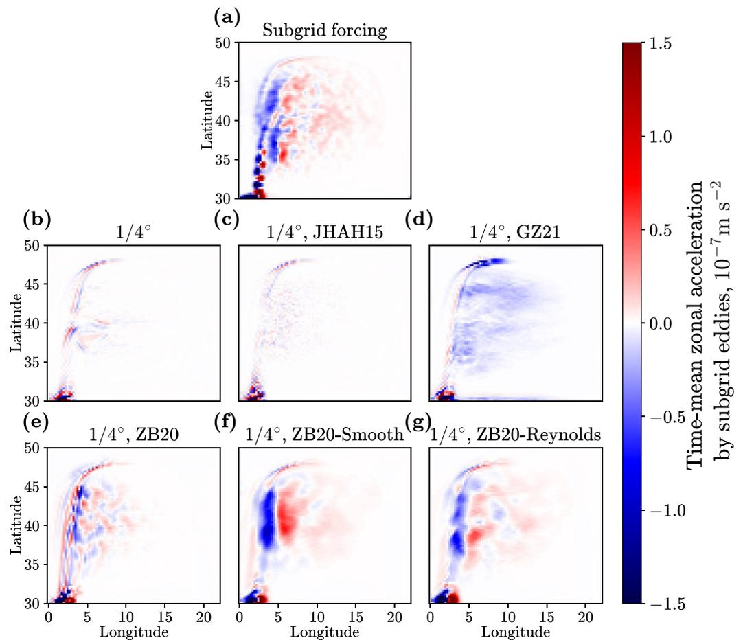
**Figure 6.** Analysis of the eddy-mean flow interaction following Hughes and Ash (2001): the 10-year mean zonal acceleration in the upper fluid layer produced by the subgrid eddies ( $\overline{\sigma_x^e}$ ). (a) The zonal component of the subgrid forcing (Equation 3), diagnosed from the  $1/64^\circ$  model by filtering and coarse-graining. Panels (b–g): the zonal acceleration, in online simulations, produced by combining each parameterization with a biharmonic Smagorinsky model.
