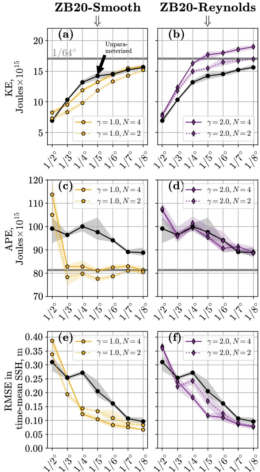
**Figure C1.** Similar to Figure 7, but showing the sensitivity to the number of the filter passes  $N$  for the filtered ZB20 parameterizations. The solid lines show the default value of the filter passes ( $N = 4$ ), and the dotted lines show a smaller value ( $N = 2$ ).
