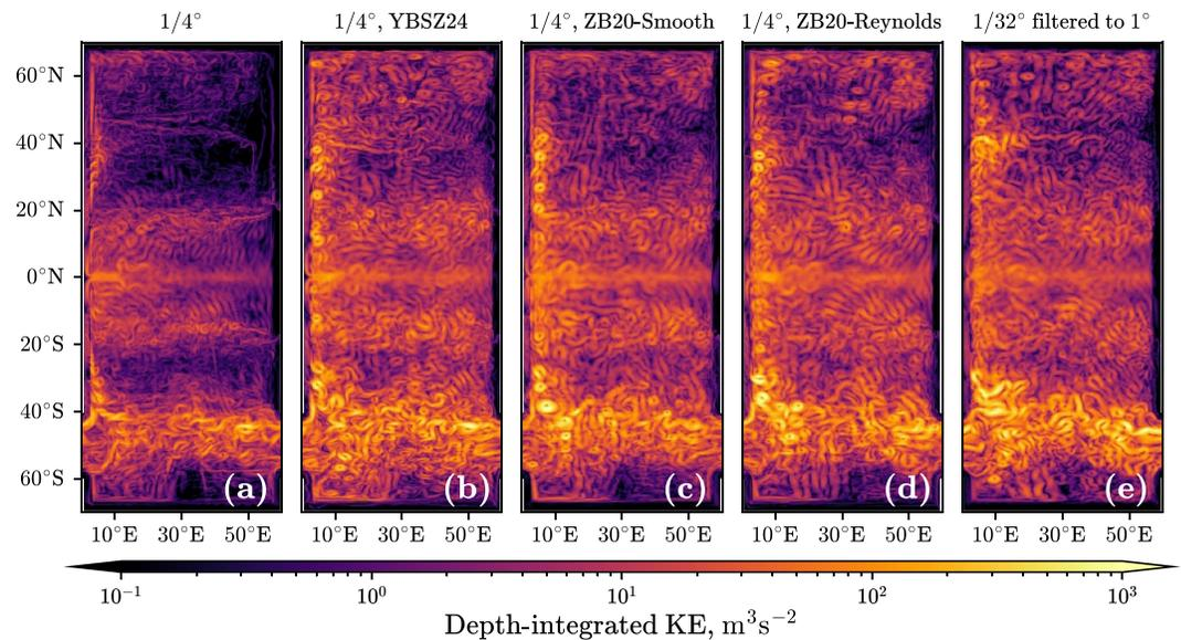
**Figure 10.** Snapshot of the depth-integrated kinetic energy. The coarse models at resolution  $1/4^\circ$ : (a) unparameterized model (biharmonic Smagorinsky), (b) Yankovsky et al. (2024) (YBSZ24), (c) and (d) filtered ZB20 parameterizations. In panel (e), we show the filtered high-resolution model  $1/32^\circ$  with filter width  $1^\circ$ .
