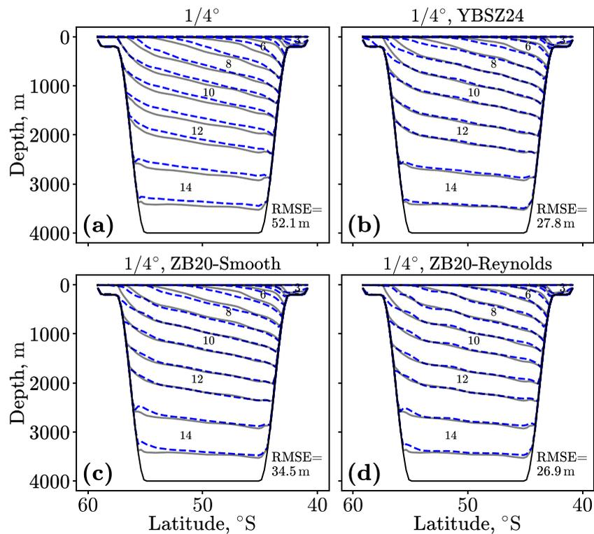
**Figure 11.** The time-mean interfaces in the meridional transect of Drake Passage (Longitude 0°E) averaged over 1,000 days. The blue dashed lines show the experiments at resolution 1/4°: (a) unparameterized model, (b) Yankovsky et al. (2024) (YBSZ24), (c) and (d) filtered ZB20 parameterizations. Gray lines show the interfaces of the high-resolution model 1/32°. The layer numbers (equal to 14, 12,...) are provided.
